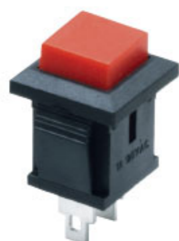
IDS-430 ON-(OFF) IDS-431 OFF-(ON) 3A 125VAC; 1A 250VAC
